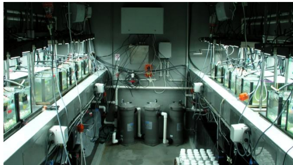
Aquarium setup for an experiment exposing corals, crustose coralline algae, foraminifera, biofilms and sea urchins to near-future CO 2 conditions.
