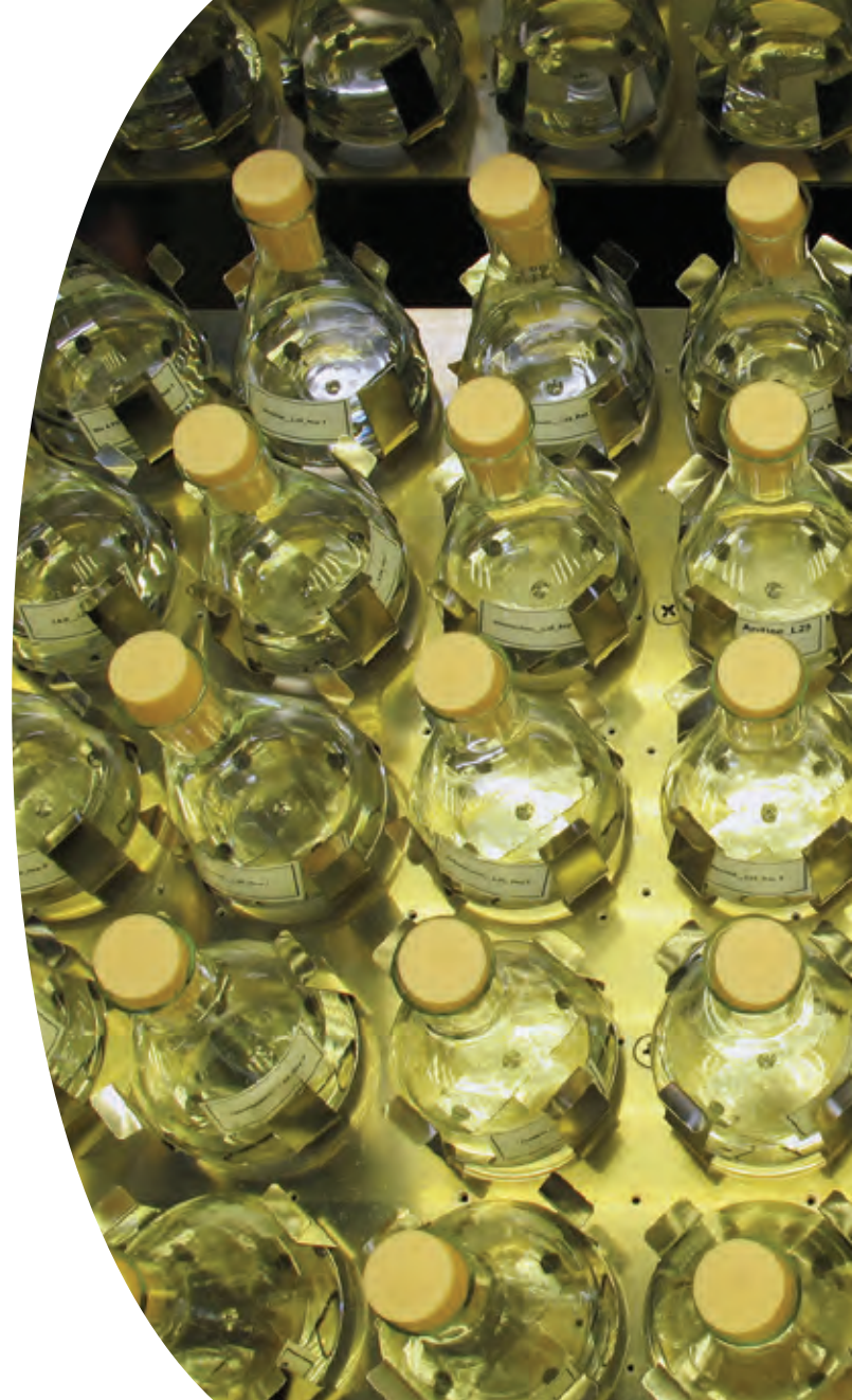
Herbicide persistence experiments using flasks in an incubator. Image: Phil Mercurio
