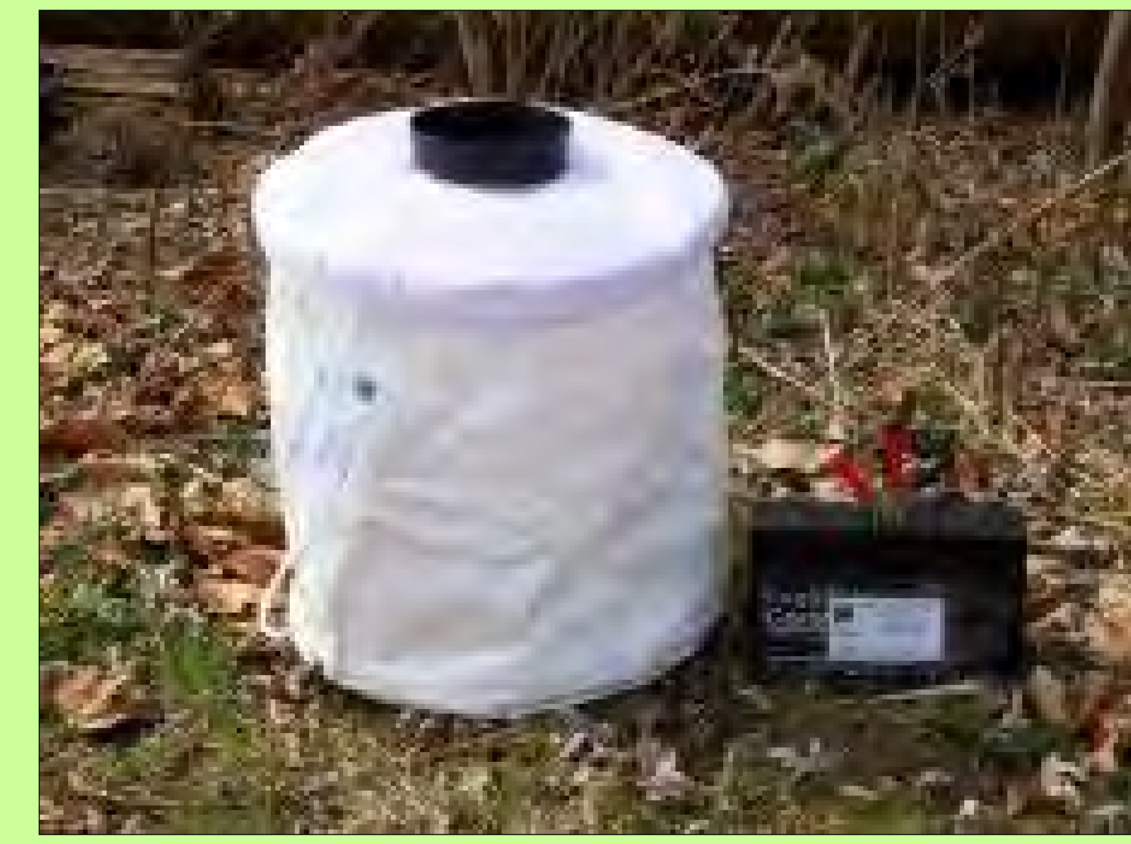
Figure 2: BGT using a power supply to operate a fan that sucks mosquitoes in
